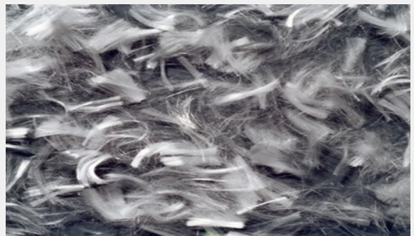
Fibrin XT BS EN 14889 Class 1a Micro Monofilament Fibre at 0.910 Kg per Cubic metre of concrete
