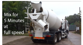
Final 5 minute mix at full speed
