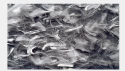
**Fibrin XT** - improves the plastic properties of the fresh concrete, resulting in better surface finsh and significantly less defects during installation of the extruded slot drain system.
