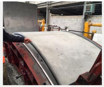
The monofilament micro synthetic fibre is added at the specified dosage during the fully automated batching process, before the concrete mix is placed and compacted into the tunnel segment moulds at the Precast Facility.
