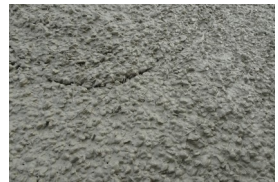
Adfil SF86 Steel fibre concrete mix
