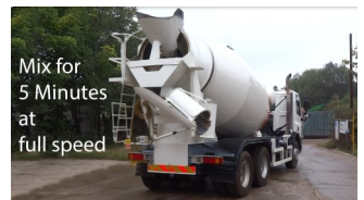
Final 5 minute mix at full speed
