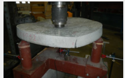
Round Panel test - ASTM C1550
